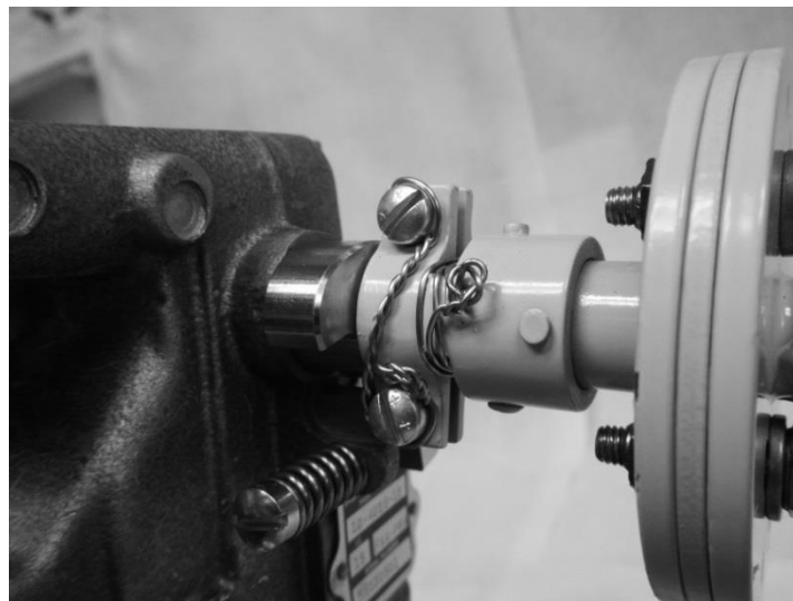
Figure 5-11e: Securing Throttle Linkage Adapter to Carburetor Stop Arm with Safety Wire
