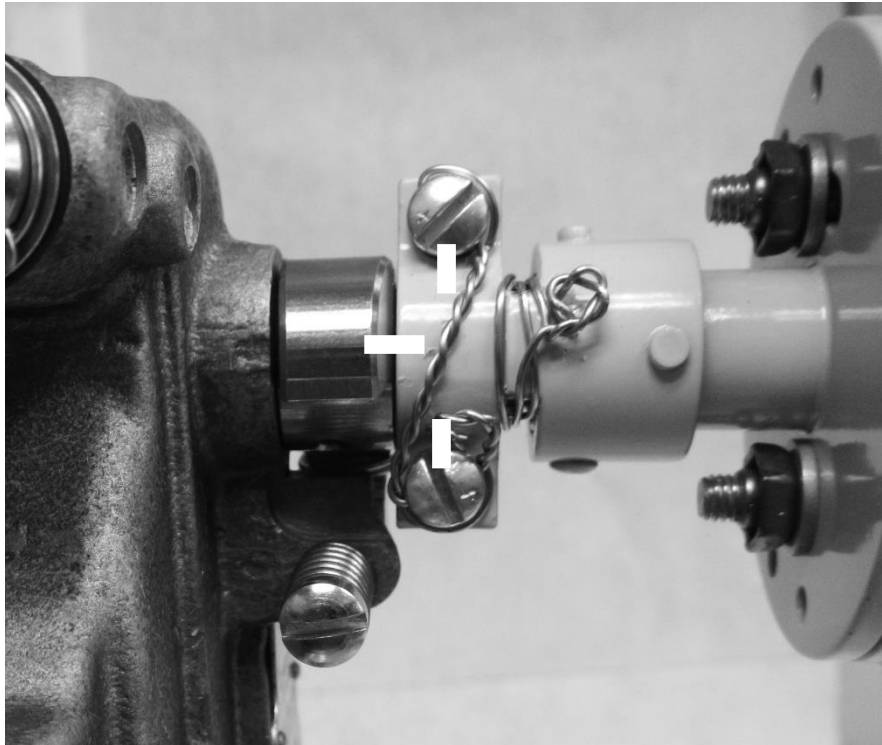
Figure 5-11f: Application of Anti-Sabotage Lacquer
